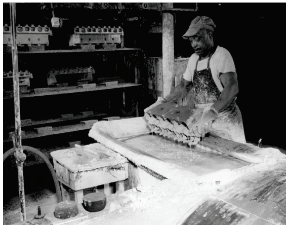
Dipping of Champion six cylinder water jacket core assembly.
